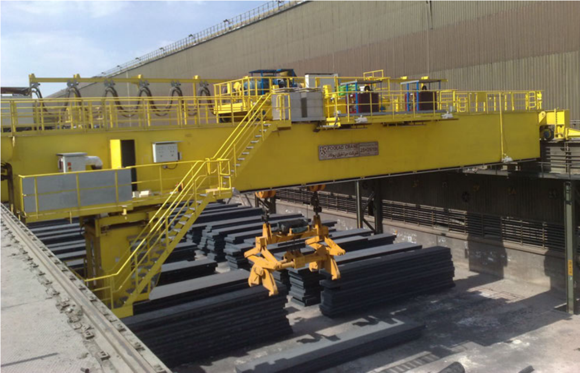
25+25(50)/10 Ton x 28m - Slab Tong Crane
