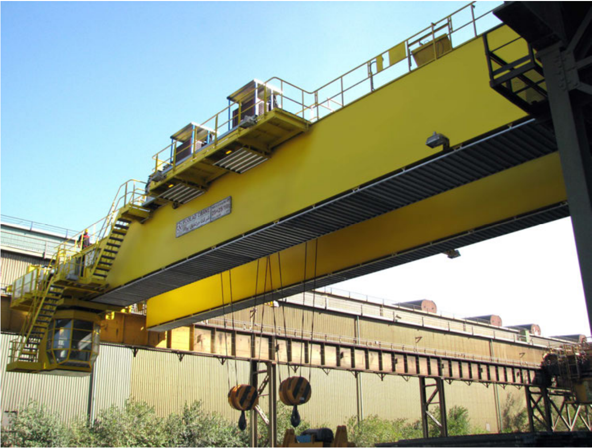
25+25(50)/10 Ton x 28m - Slab Tong Crane
