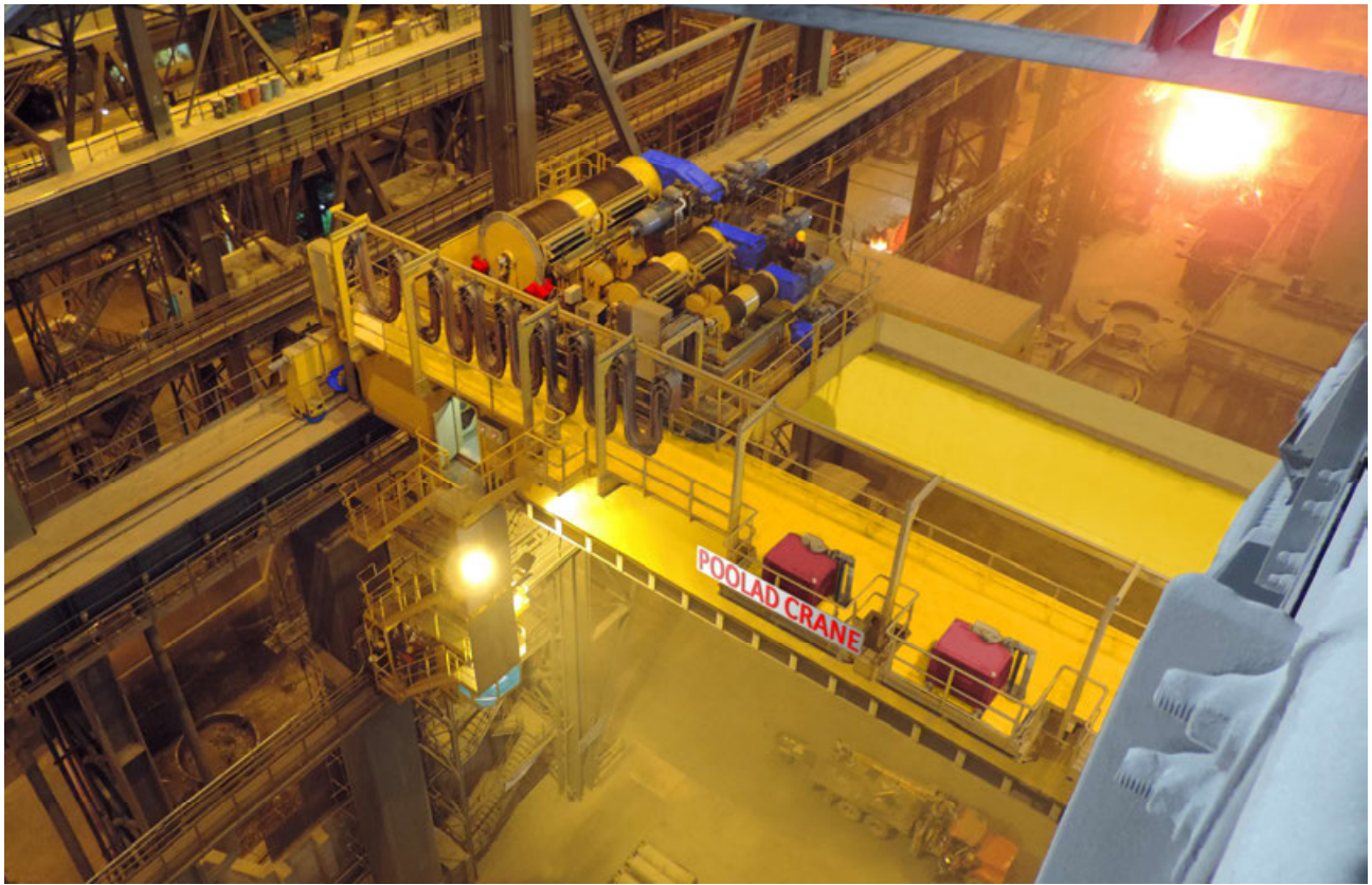
Scrap Charging Crane 110/40/10 Ton x 30 meters
