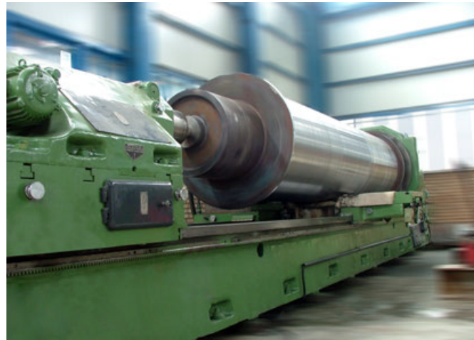
Heavy Lathe Machine Machining line For manufacturing of heavy duty cranes drums
